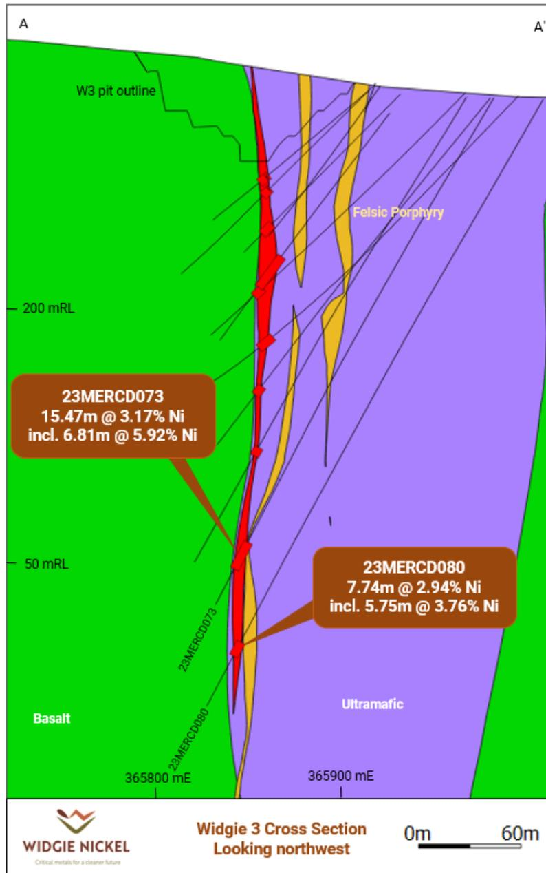
Figure 6 23MERC073 and 23MERC080 drill section
